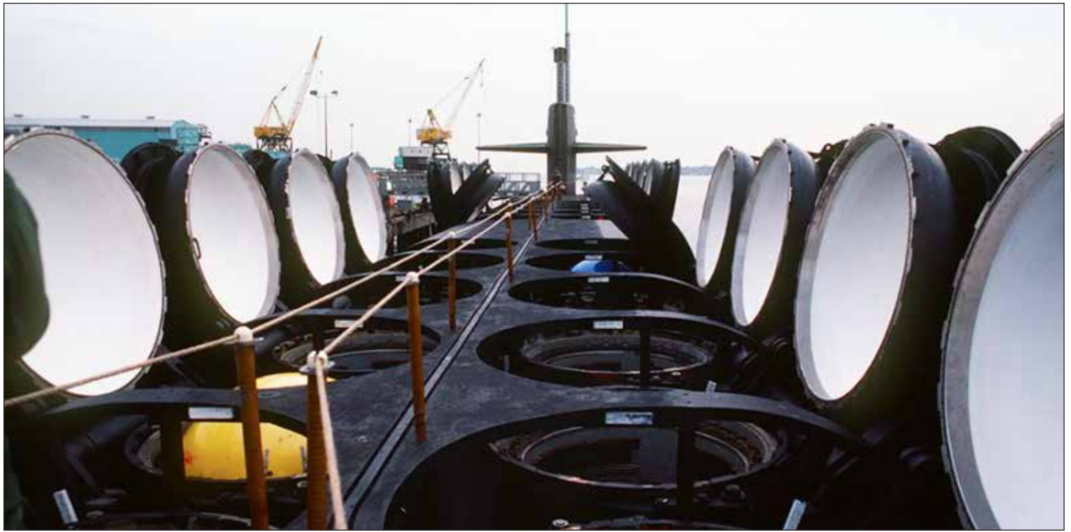
U.S. Navy ballistic missile submarine Ohio with her missile tubes open during pre-commissioning activities, Feb. 6, 2001. (U.S. Navy photo.)
